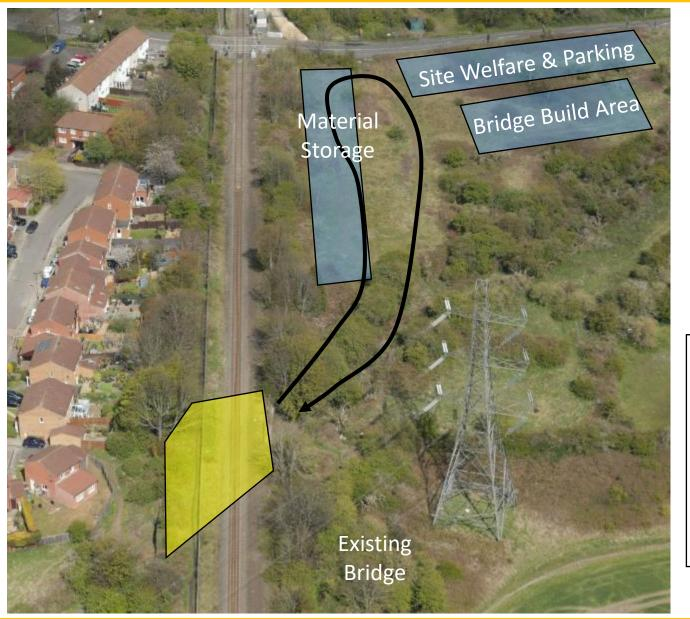
Bridge area to be excavated as required by design and moved to North end of material storage area along designated route shown.
